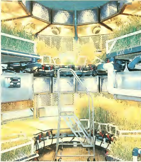
A CELSS plant growth experiment conducted within the Breadboard biomass production chamber.
